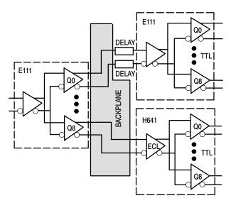
Figure 9. Mixed ECL and TTL Distribution
