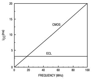
Figure 6. ICC/Gate vs Frequency Comparison
