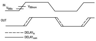
Figure 3. V<sub>BB</sub> Induced Duty Cycle Skew
