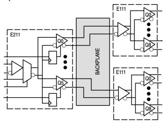
Figure 7. ECL Clock Distribution Tree
