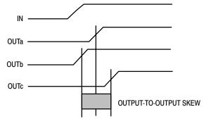
Figure 2. Output-to-Output Skew
