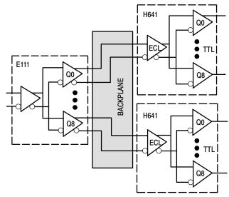
Figure 8. ECL to TTL Clock Distribution
